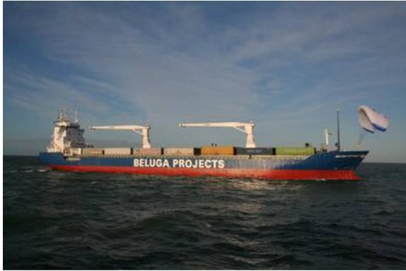
Fig.6: Towing kite harnessing wind energy, source: [www.skysails.de](http://www.skysails.de)
