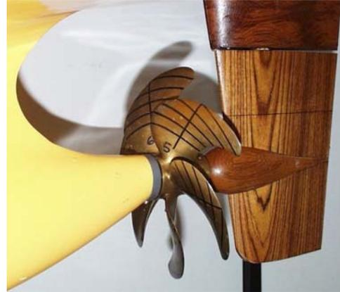
Fig.2: Twisted rudder with Costa bulb, source: [www.hsva.de](http://www.hsva.de)
