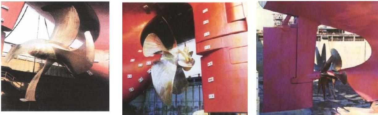
Fig.3: Improving propulsion: CLT propeller (left), PBCF (center), Grim vane wheel (right)
